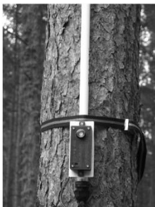
Fig 1: Forest fire detection hydrogen sensor implementation
